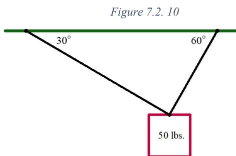
There are three forces working on the speaker; the weight of the speaker, which we will call  $\mathbf{w}$ , that pulls the speaker directly downward, and the forces on the cables, which we will call  $\mathbf{T}_1$  and  $\mathbf{T}_2$  (for ‘tensions’) acting upward at angles  $60^\circ$  and  $30^\circ$ , respectively. Following is a corresponding vector diagram.
