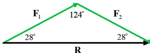
The measure of the angle between vectors  $\mathbf{F}_1$  and  $\mathbf{F}_2$  is  $180^\circ - 28^\circ - 28^\circ = 124^\circ$ . We have been given the magnitude of the resultant vector,  $\mathbf{R}$ , which is 4,400 pounds. Our goal is to find the tensions in the tow lines, or the magnitudes of  $\mathbf{F}_1$  and  $\mathbf{F}_2$ . We can use the Law of Sines here.
