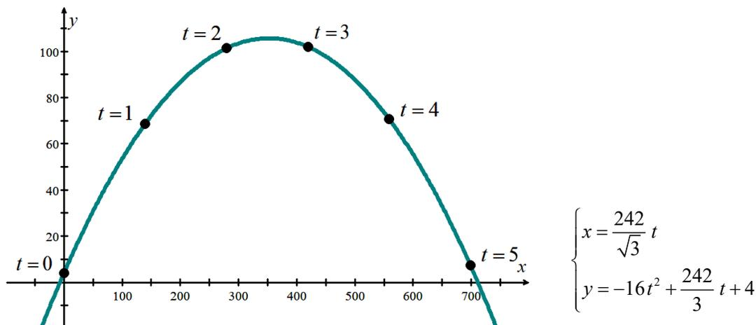
To determine how far the baseball will travel horizontally, we look for the time when the height of the ball is zero. The time is found by setting  $y$  equal to zero:  $y = -16t^2 + \frac{242}{3}t + 4 = 0$ . After applying the quadratic formula,
