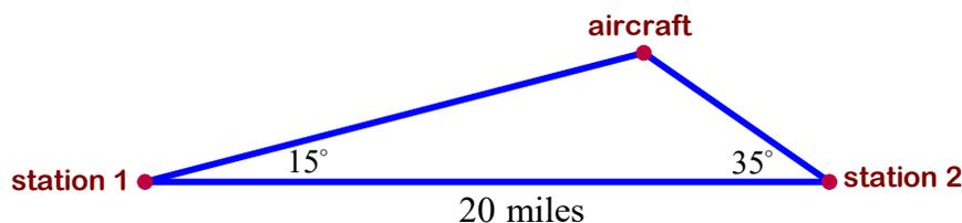
The angle of elevation measured by the first station is 15 degrees, whereas the angle of elevation measured by the second station is 35 degrees. Find the altitude of the aircraft and round your answer to the nearest tenth of a mile.
