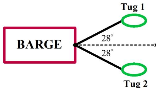
Each tow line connecting the barge to one of the tugboats makes an angle of  $28^\circ$  with the path of the barge. Find the tension (magnitude of the ‘pulling’ force) in the tow lines if the resultant force on the barge has a magnitude of 4,400 pounds.
