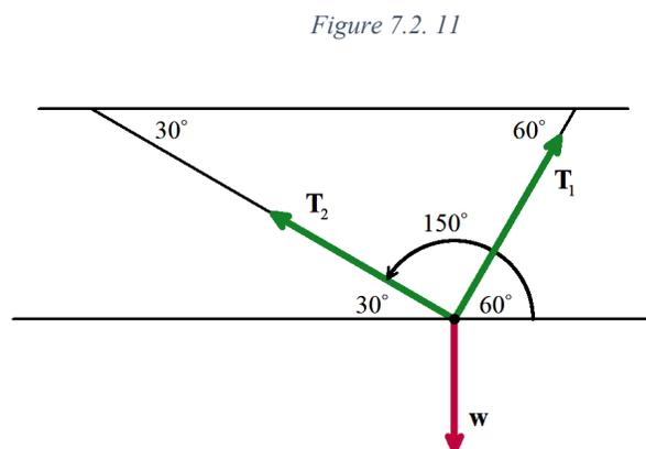
We are looking for the tensions on the cables, which are the magnitudes  $\|\mathbf{T}_1\|$  and  $\|\mathbf{T}_2\|$ . Since the speaker is stationary,<sup>8</sup> we must have  $\mathbf{w} + \mathbf{T}_1 + \mathbf{T}_2 = \mathbf{0}$ . Viewing the common initial point of these vectors as the origin and the horizontal line through this point as the  $x$ -axis, we find component representations for the three vectors involved.
