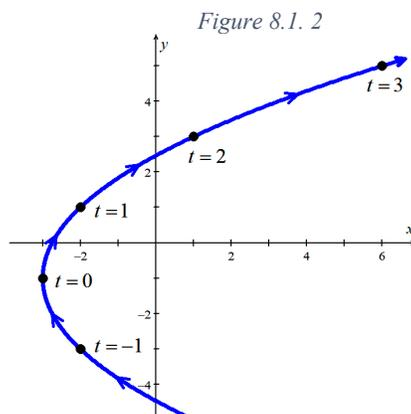
Notice that as  $t$  increases, a particle whose position is given by these parametric equations moves along the curve in the direction of the arrows.
