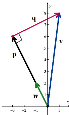
From the definition of vector arithmetic,  $\mathbf{p} + \mathbf{q} = \mathbf{v}$ , so that  $\mathbf{q} = \mathbf{v} - \mathbf{p}$ . In the case of **Example 7.3.4**, with  $\mathbf{v} = \langle 1, 8 \rangle$  and  $\mathbf{p} = \langle -3, 6 \rangle$ , we find  $\mathbf{q} = \langle 1, 8 \rangle - \langle -3, 6 \rangle = \langle 4, 2 \rangle$ . Then
