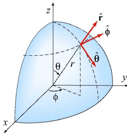
**Figure 9A.2** Spherical coordinates
