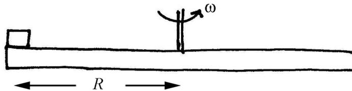
Figure 9.14 Coin on Rotating Turntable
