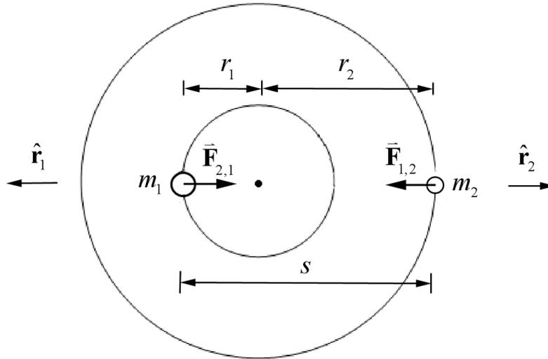
**Figure 9.7** Force diagrams on objects 1 and 2
