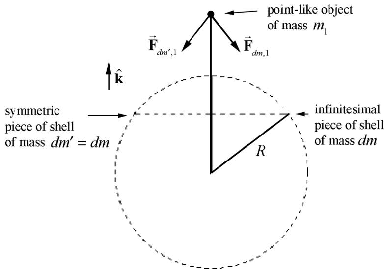
**Figure 9A.5** Symmetric cancellation of components of force
