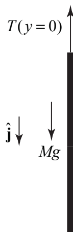
Figure 8.27 Force diagram on rope
