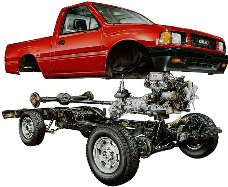
A mechanical assembly is represented as a **tree** of subassemblies down to individual parts.
