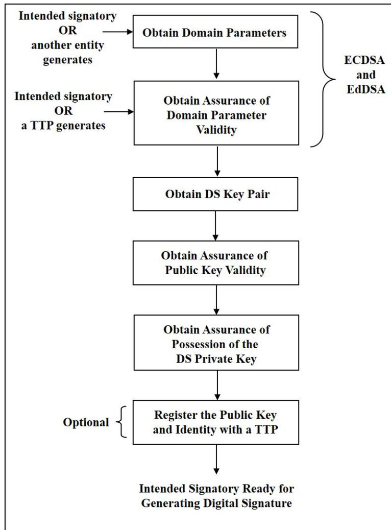
**Figure 2: Initial Setup by an Intended Signatory**
