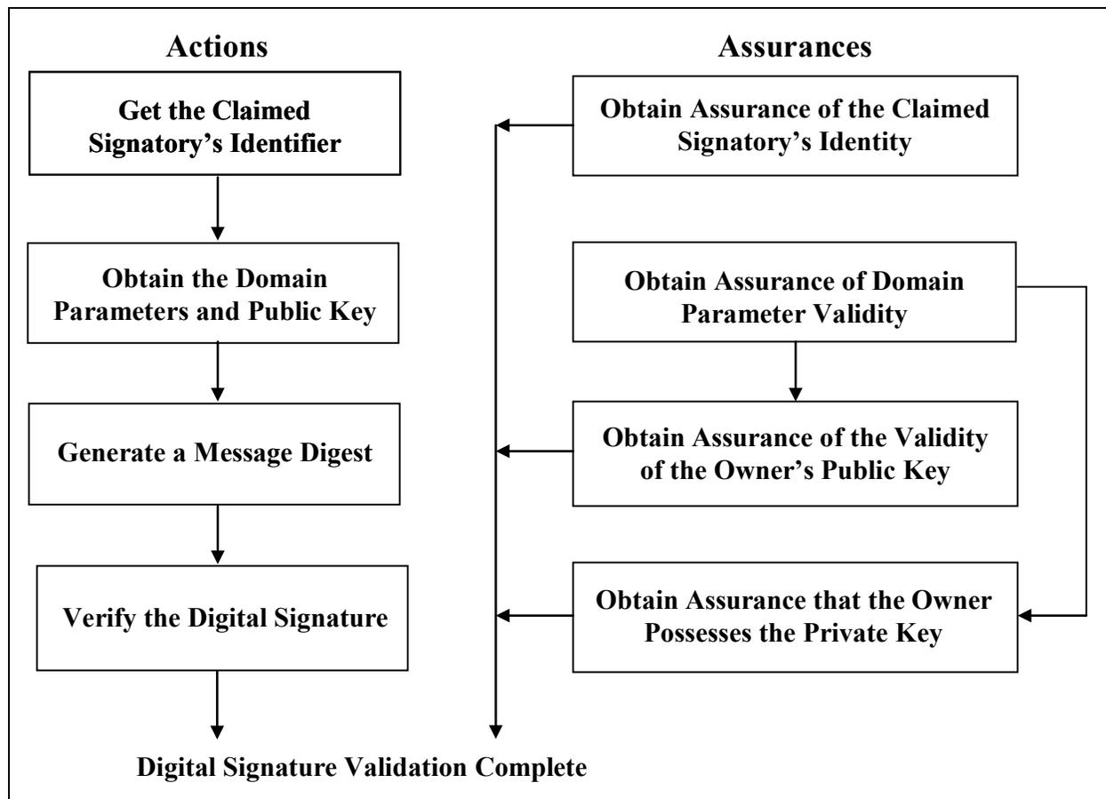
Figure 4: Digital Signature Verification and Validation<sup>6</sup>
